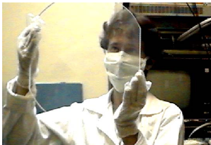
Fig. 2.2. Installations for growing large-aperture nonlinear optical crystals in IAP RAS (left) and element for frequency conversion of superintense optical radiation
