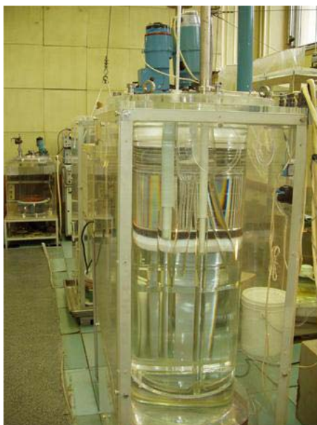
Fig. 2.2. Installations for growing large-aperture nonlinear optical crystals in IAP RAS (left) and element for frequency conversion of superintense optical radiation
